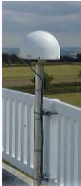
CORS permanently mounted GPS base receiver.
