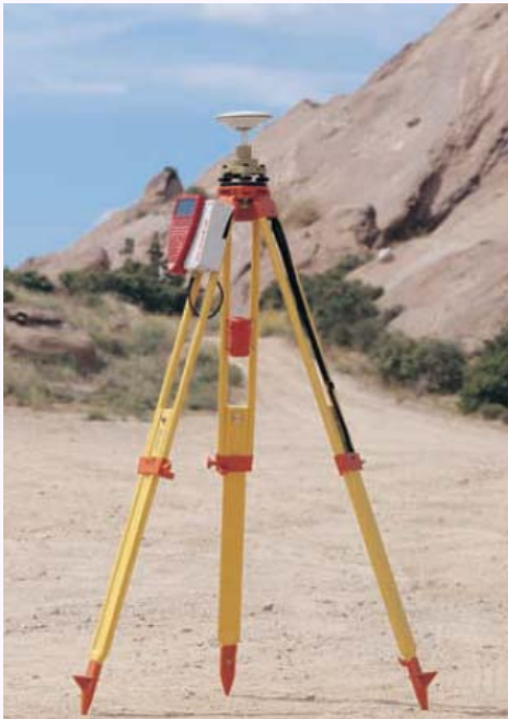
GPS base receiver mounted on a known position, but capable of moving from point to point as needed.
